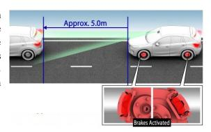
We can include Dynamic Brake System and Crash Imminent Braking as functions of the AEB system.
