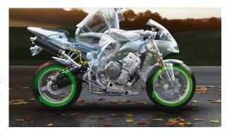
serves furthermore to prevent the front wheel from moving up when accelerating under full power (Anti Wheelie Control).
