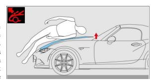
designed to rise in a crash involving VRUs to soften the crush, absorb the head impact energy, and reduce the severity of the injury. Several manufacturers are developing these systems, which are often combined with external airbags.
