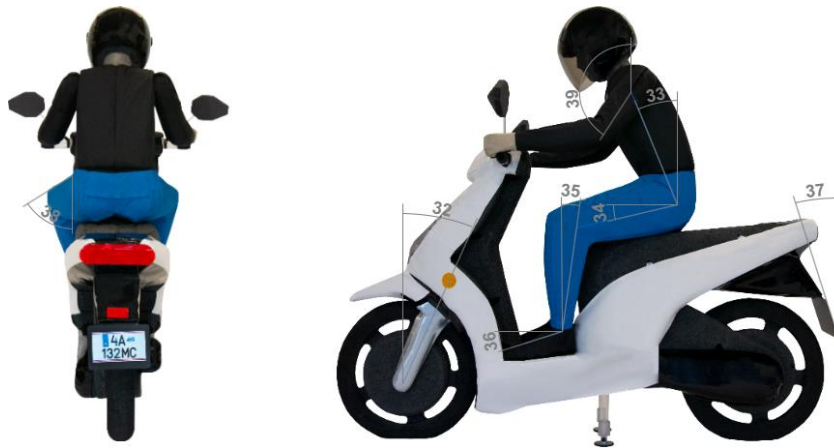
Figure 3 Scooter target dimensions and dummy posture
