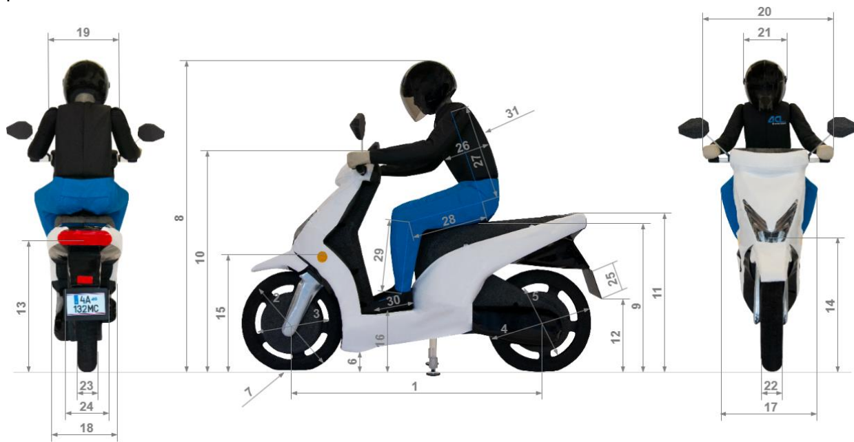
Figure 2 Scooter target dimensions and dummy posture
