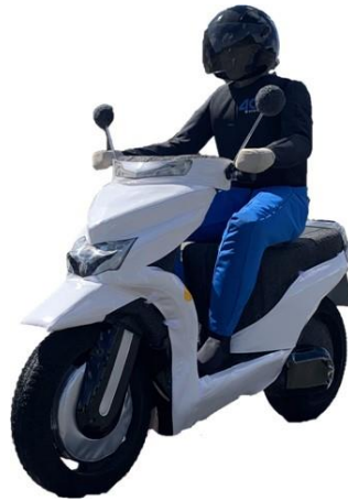
Figure 25: AMT - ASEAN Motorcycle Target dummy
